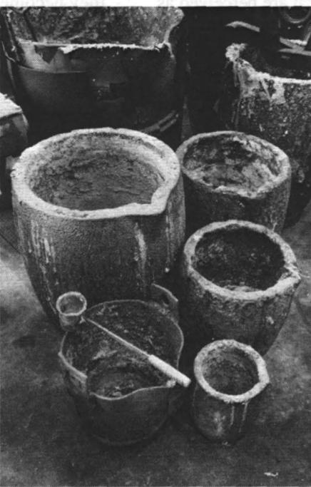
Most of the metals cast at Sandia's Foundry, Pattern, and Heat Treating Div. 7473-5 are aluminum or copper alloys. Steel is currently melted at Dept. 1830's Area III facility. Aluminum alloys made at Sandia usually come in three varieties — one variety is made of seven percent magnesium, another is seven percent zinc, and a third is seven percent silicon. Copper alloys include bronze and brass. The section accepts work orders from other government agencies as well as Sandia.
